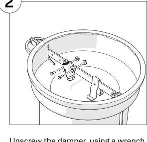
Unscrew the damper, using a wrench.
