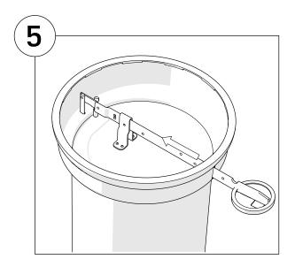
Slide the new pedal in and realign the lidstop.
