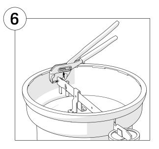
Attach the new rivets, using a bit and pliers.
