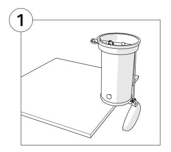
Place the bin upside down, with the lid open, on a table for an easier working position.
