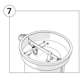
Reattach the damper, using the two cutouts closest to the middle.
