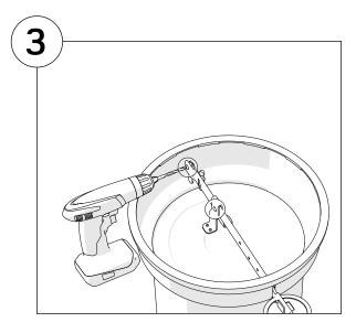
Drill out the two rivets, using a drill.
