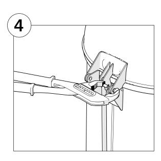
Use pliers and a screwdriver bit to expand each revit.
