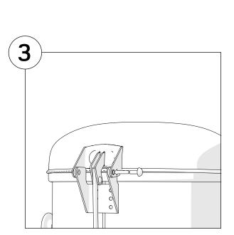
Change the lid, align the holes and insert the new revits.
