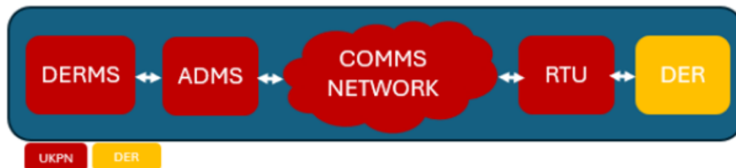
Figure 2-1 Communication hierarchy for a Flexible Connection
