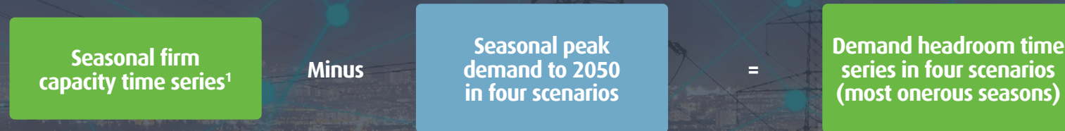
Figure 7 High-level approach to estimating unused capacity for demand per substation
