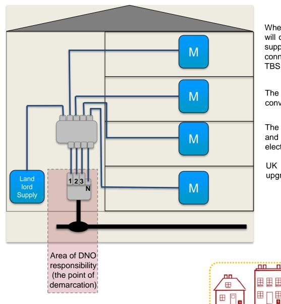
When the conversion takes place the customer will often use the supply for a temporary builders supply; please note that an RCD will be required, connected to the customers earth stake for the TBS: it will provide a TT supply.
