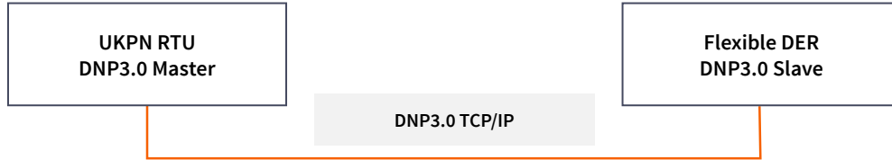
Figure 14 Flexible Connection communications protocol
