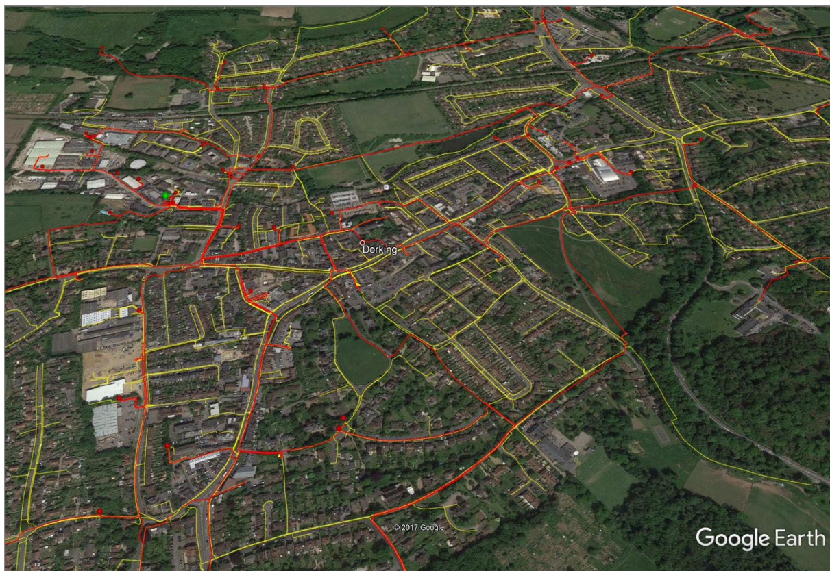
Figure G-1 – HV and LV Cable Network
