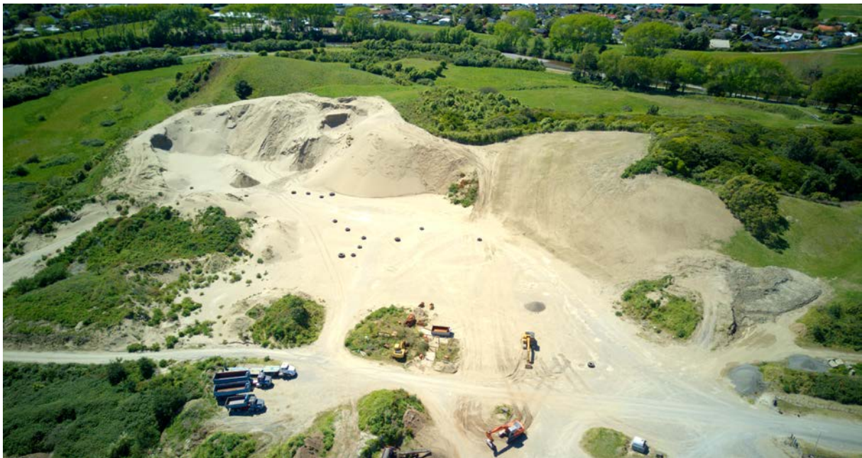
Figure 2.5 Quarry at Otaihanga on the Kāpiti Coast extracting sand from an old sand dune inland from the modern-day coast. (Photography by Matthew Hill, GNS Science.)
