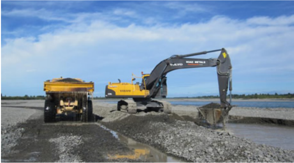
Figure 2.4 Waimakariri Quarry operating near the active river in Christchurch harvesting river gravel material for local roads, drainage and concrete components. (Photograph courtesy of Road Metals Ltd.)
