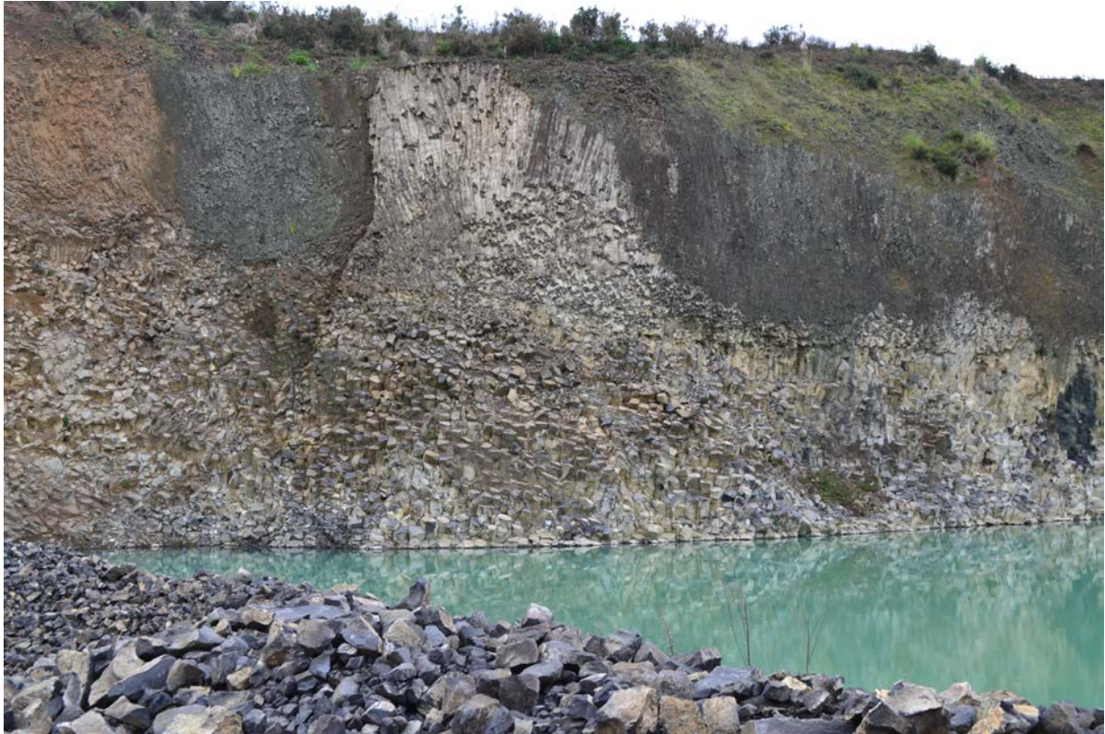
Figure 2.2 Pukekawa Quarry near the Waikato River extracting basalt hard rock aggregate. Basalt columnar jointing visible in exposed face. (Photography by Matthew Hill, GNS Science.)
