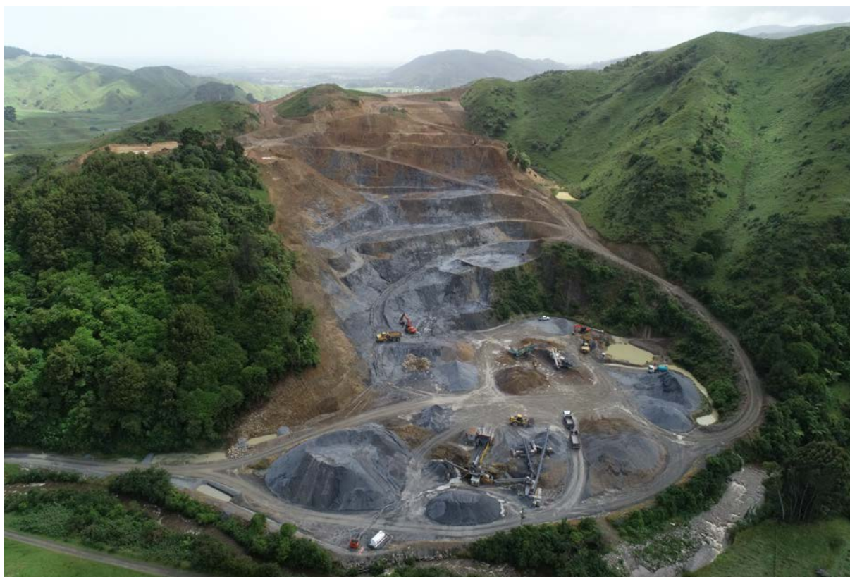
Figure 2.1 Waitohu Quarry near Otaki extracting greywacke hard rock aggregate with the contact between the weathered (brown) and un-weathered (blue-grey) material visible. (Photography by Matthew Hill, GNS Science.)
