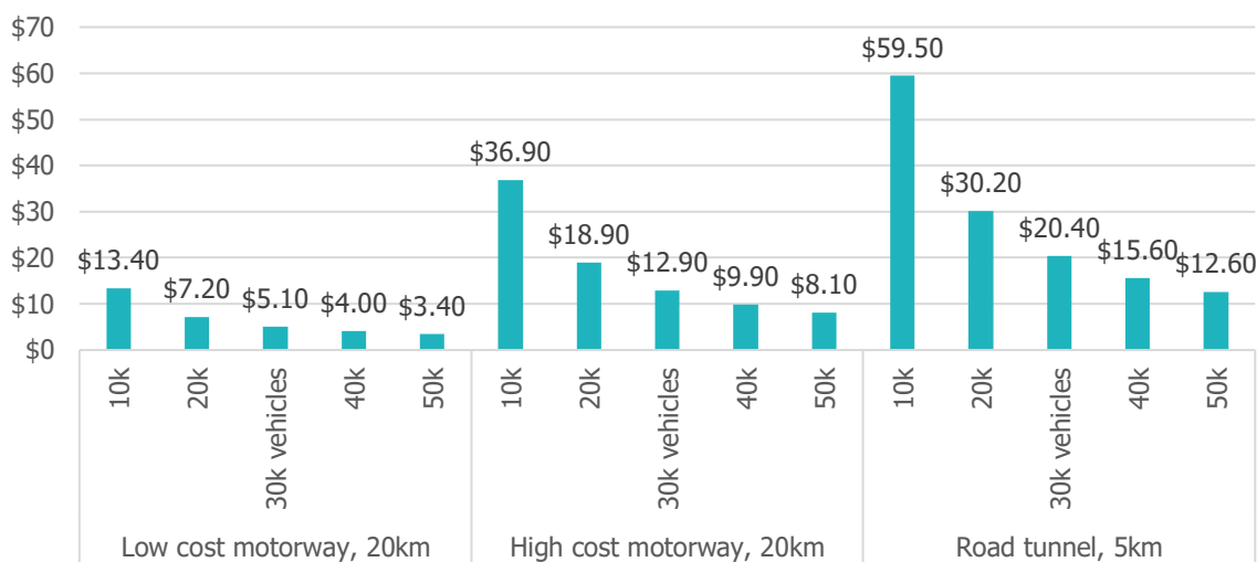
Figure 9: Required light vehicle tolls to achieve full cost recovery for new roads
