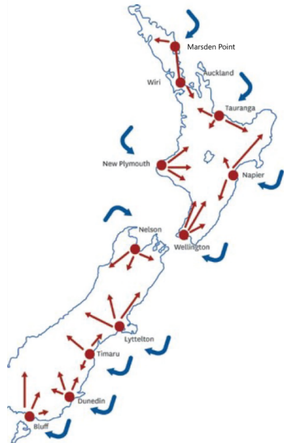
Figure 6: National fuels supply chain (source: National Infrastructure Vulnerability Assessment, 2022). Note that blue arrows denote fuel shipments; red arrows show general direction of trucked and piped supply from ports.
