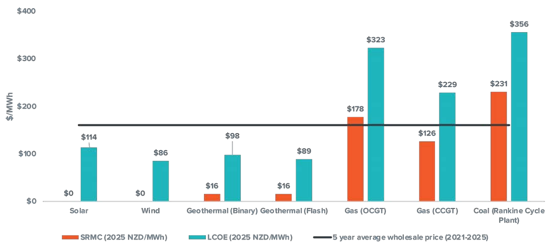
Figure 8: Estimates of short run marginal costs and levelised cost of electricity, by type of plant, year 2025
