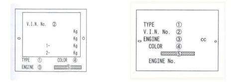
With the Type 1 plate, the VIN is usually on the third line and comprises of a 17-digit alpha-numeric string. On the Type 2 plate, the VIN is normally an 11-digit alpha-numeric string. The engine number on the plate only shows the engine type: the actual engine number is stamped on the engine block. Locations vary, so guidance can be sought from your vehicle handbook or dealer.
