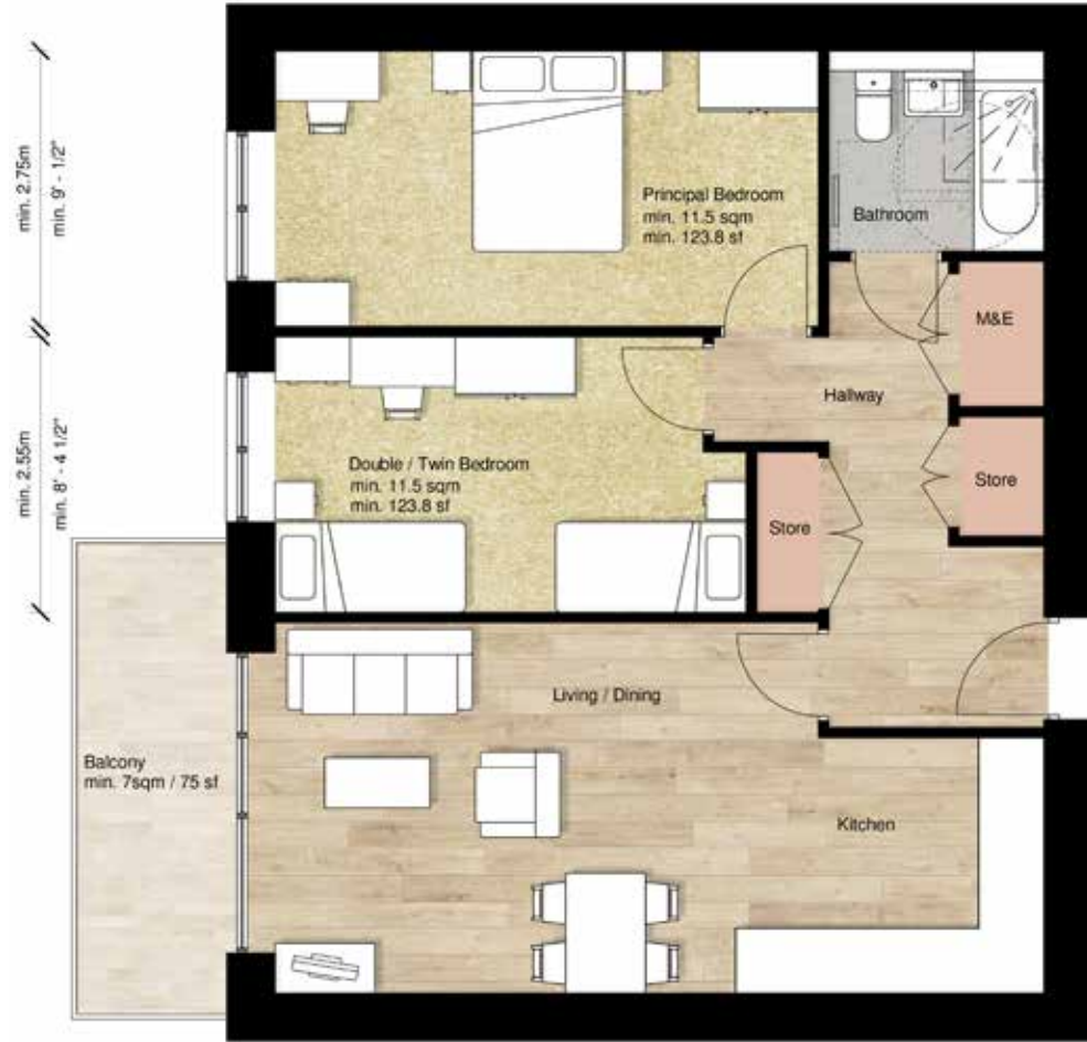
TYPICAL UPPER FLOOR Min. Area: 70 sqm / 753 sf Min. Storage Area: 2 sqm / 21.5 sf
