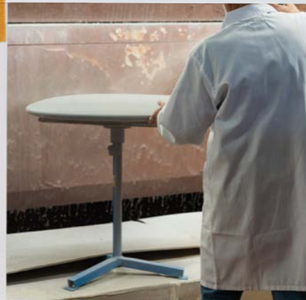
Semi-dry, a specially developed glaze is spray-painted by hand
