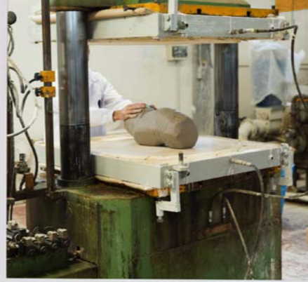
Clay is pressed into form
