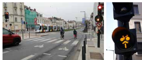
Example of traffic lights allowing bikes to pass at the same time alongside light rail vehicles
