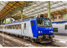
Figure 5: Z2 EMU (electric multiple unit)
