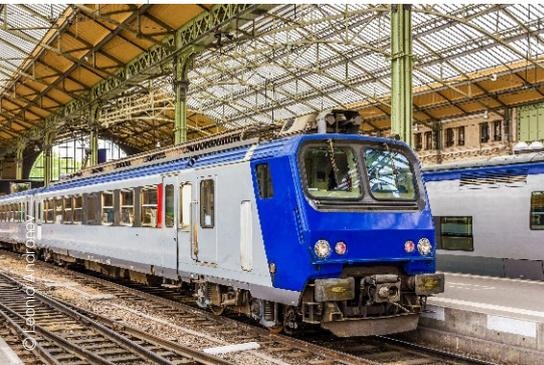
Figure 5: Z2 EMU (electric multiple unit)
