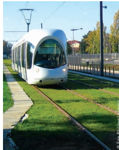
Lyon T3 - RhôneExpress, embedded grass-covered ballast track, mixed urban and railway section
