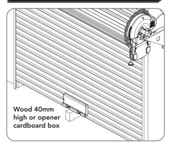
WARNING! If the door fails these tests, put the opener into manual mode, only operate the door by hand and call for service.
