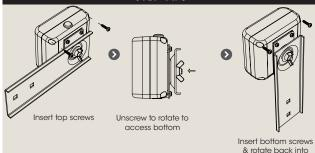
& rotate back into position & tighten
